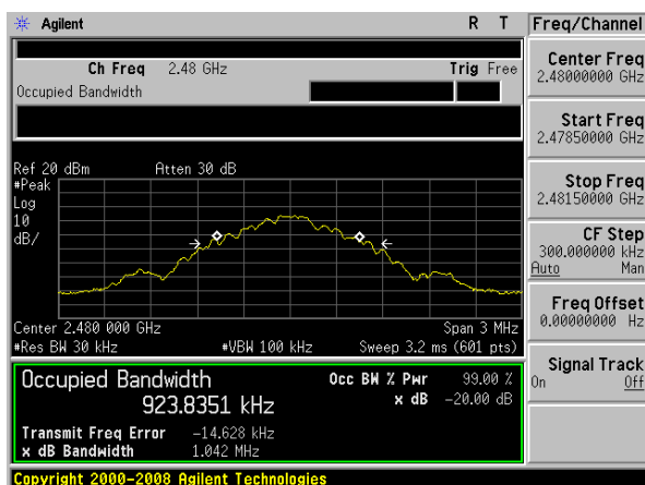
20dB Bandwidth plot on channel 78 (1Mbps)
