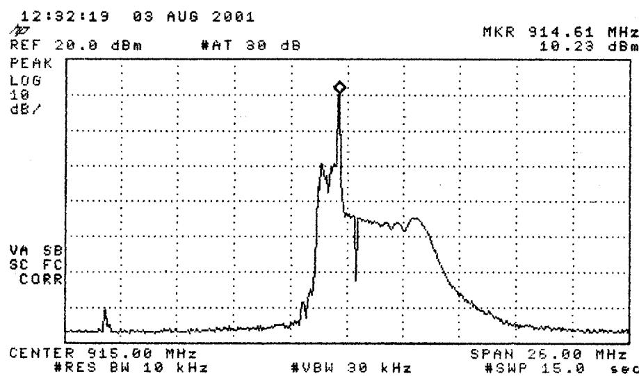
Figure 6.3. Band-edge emissions of the DUT (repeated pulsed emission).
