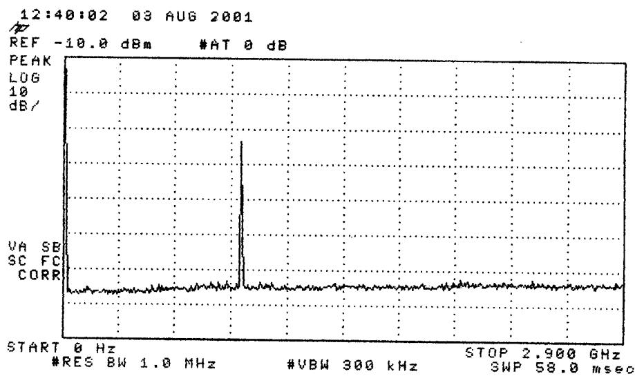
Figure 6.2. Emission spectrum of the DUT (repeated pulsed emission). The amplitudes are only indicative (not calibrated).
