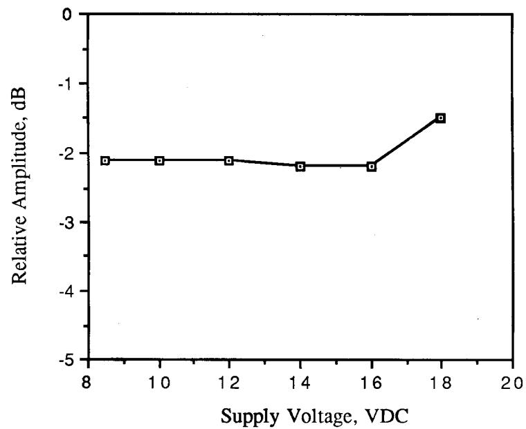
Figure 6.3. Relative emission at fundamental vs. supply voltage.
