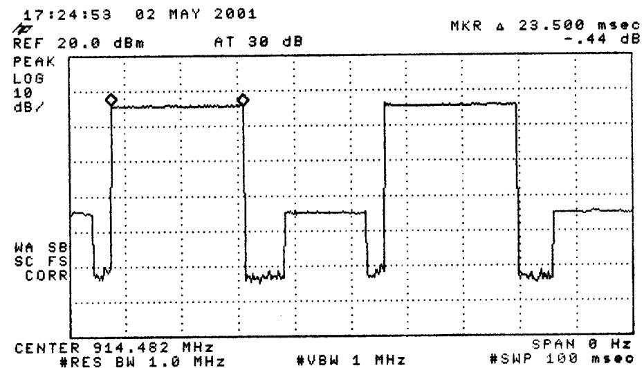
Figure 6.1. Transmissions modulation characteristics: (top) pulse period, (bottom) pulse width.
