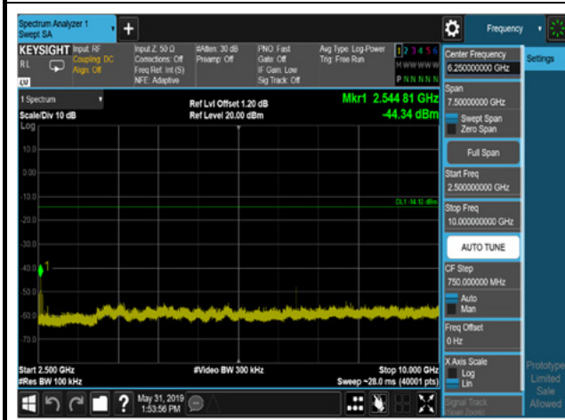
8DPSK,2480MHz,3DH5,Plot 1,Band Edge
