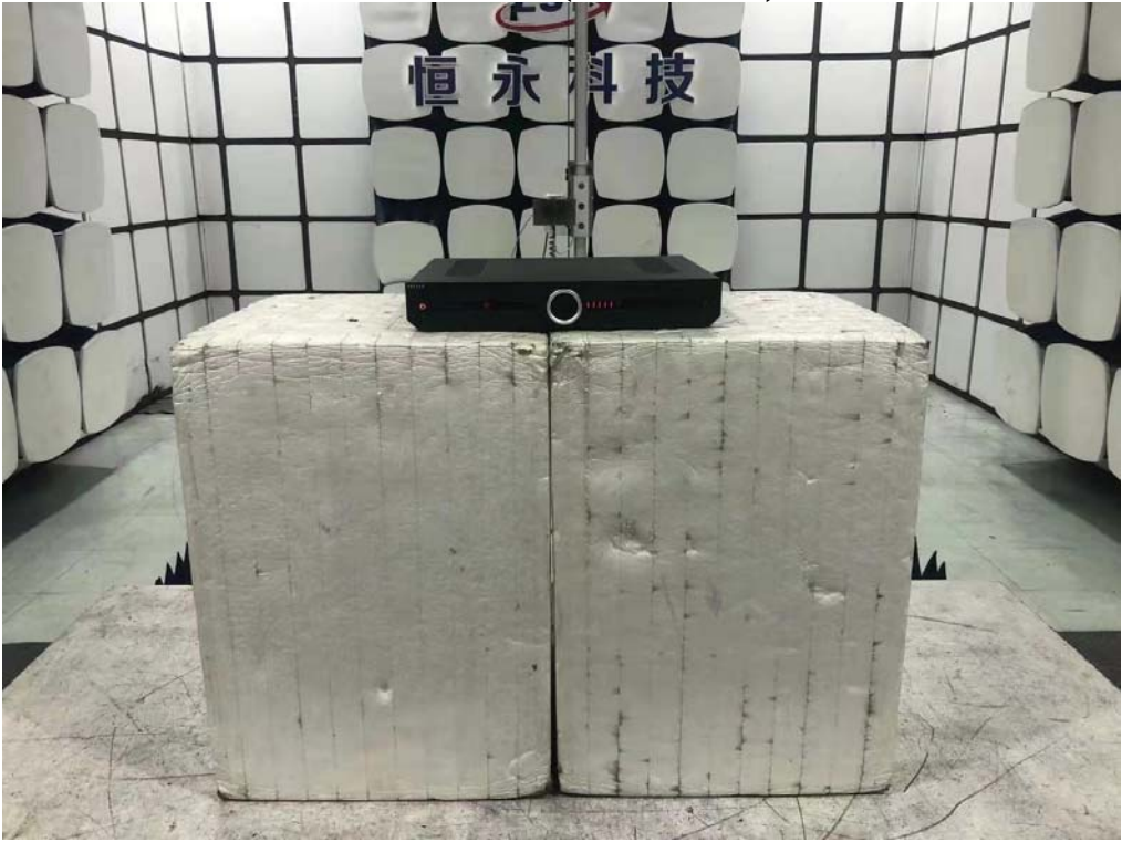
Radiated Test (Above 1GHz)
