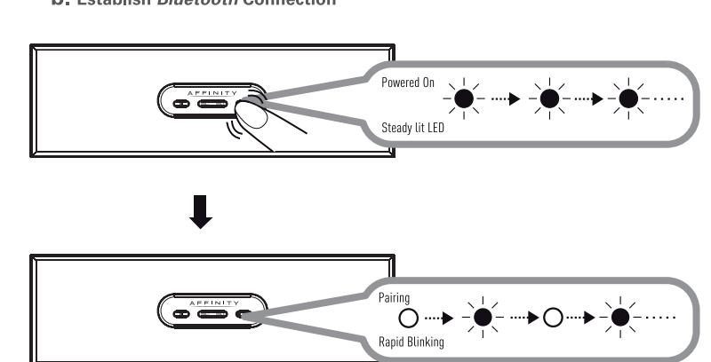
The LED status indicator will lit steady indicating the speaker is currently ON. To allow pairing to other Bluetooth devices, Press and Hold the CONNECT button for 3 seconds. Release when 2 beep tones are heard with the LED status indicator blinking rapidly.
