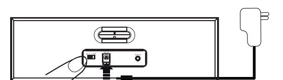
Attach the DC cord to the DC IN and flick the Power switch to ON position
