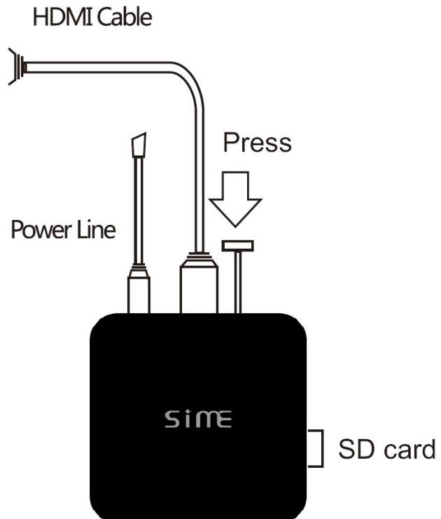
7.5 You can stop pressing the reset button until you see the android robot. And use the remote to choose "apply update from EXT" → choose "Update from SD card" → Choose "xxx.zip (the upgrade package file)" and press OK.
