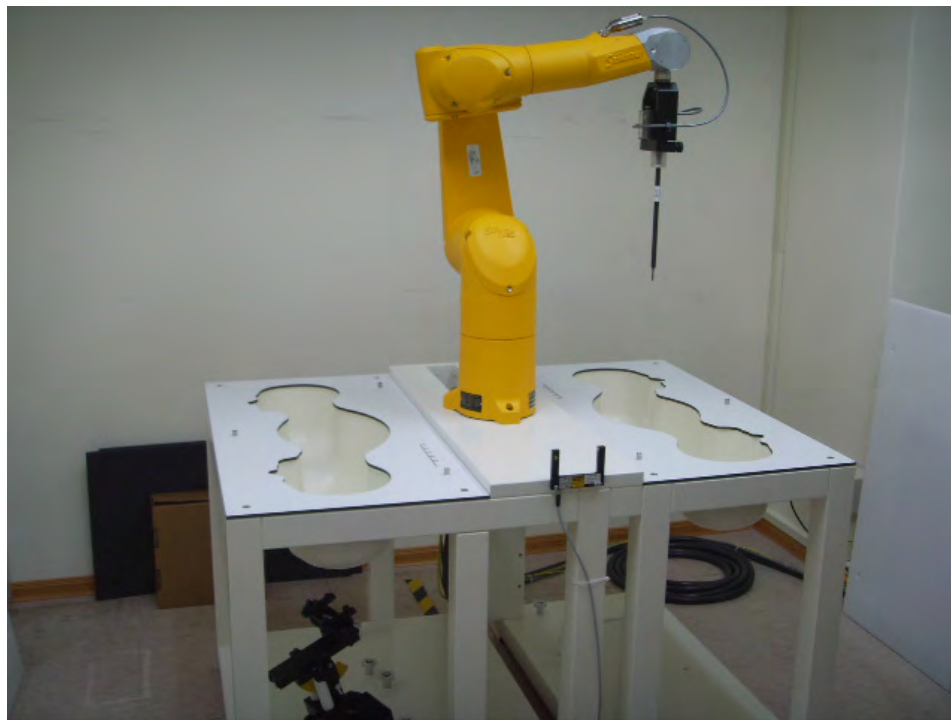
Fig.1 Photograph of the SAR measurement system
