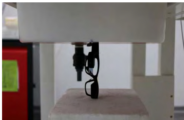
Fig.4 Position the outside of the arm against the phantom(Plot 2)
