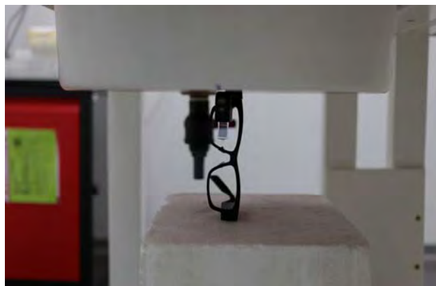
Fig.3 Position the outside of the arm against the phantom(Plot 1)
