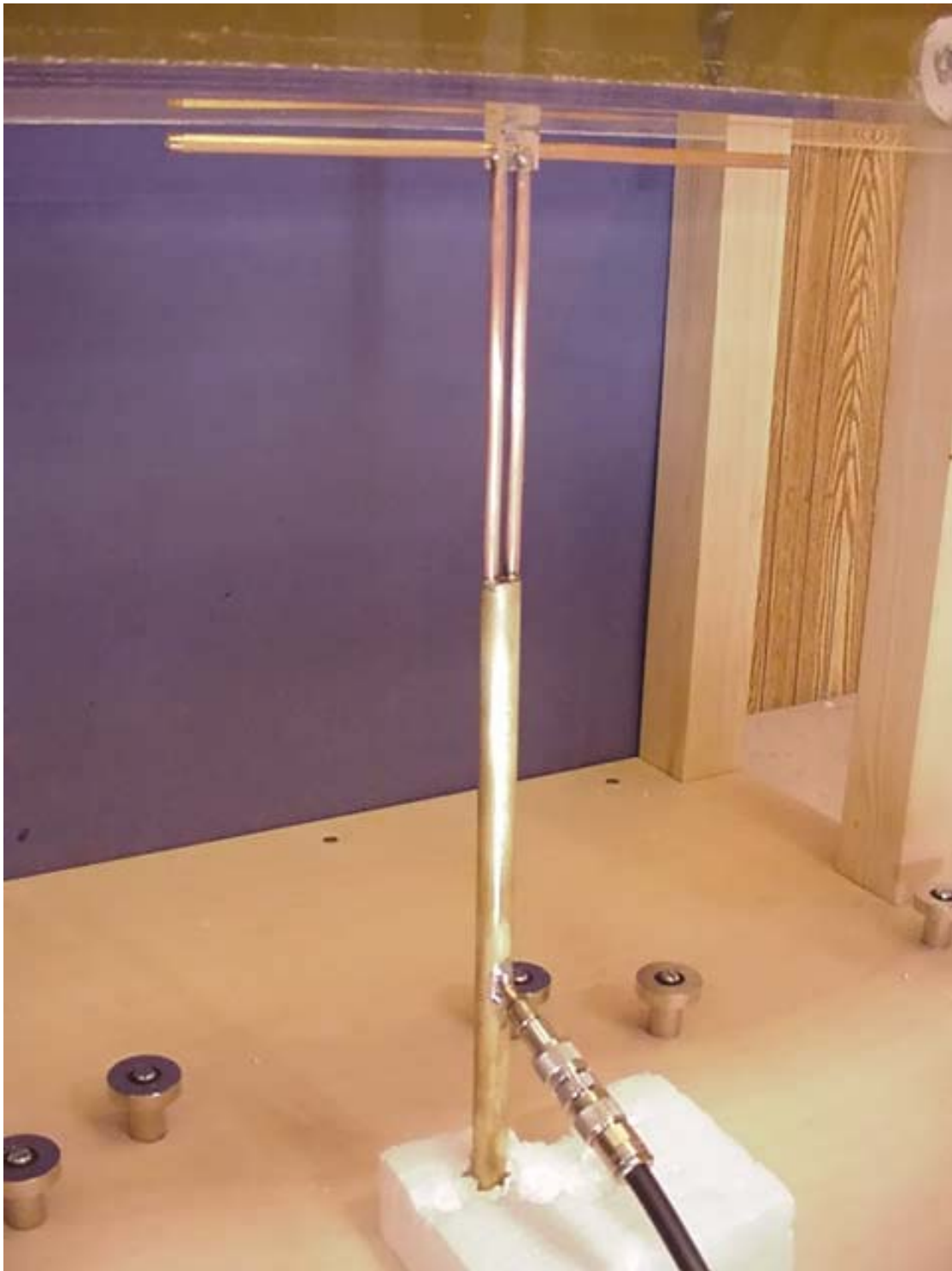
450MHz Dipole Calibration Photo
