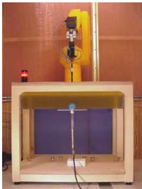
DASY3 SAR Measurement System with small planar phantom DASY3 SAR Measurement System with large planar phantom
