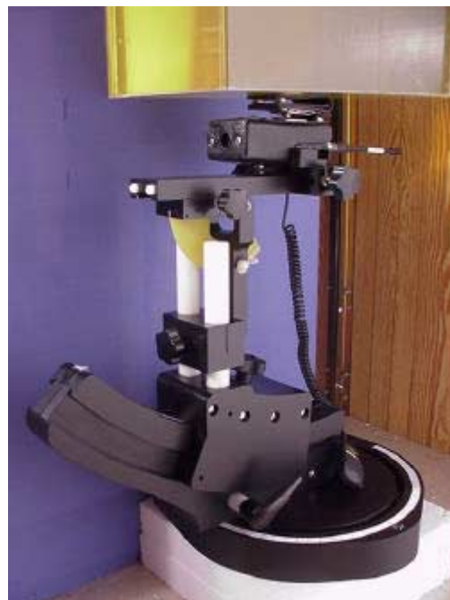
Body SAR Test Setup with small planar phantom
