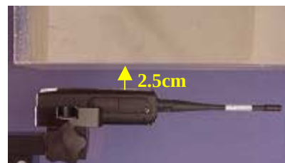
Face-held SAR Test Setup 2.5cm Separation Distance
