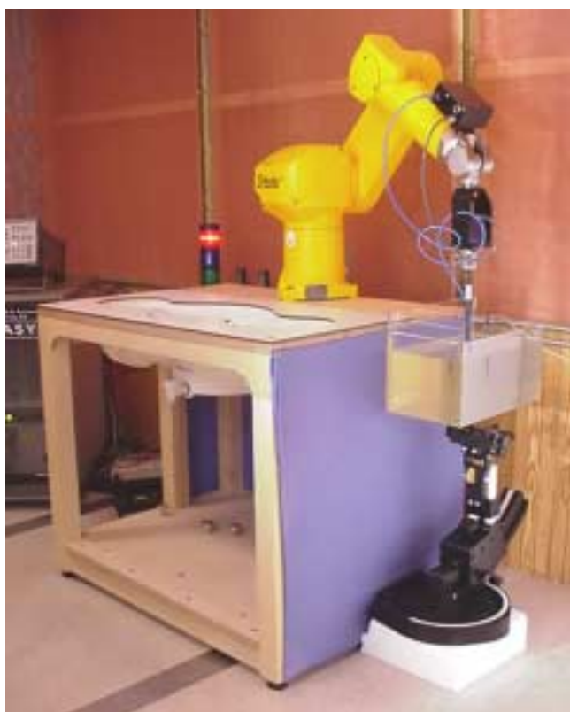
DASY3 SAR Measurement System with small planar phantom DASY3 SAR Measurement System with large planar phantom
