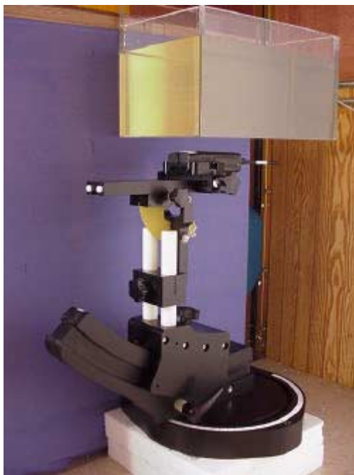
Face SAR Test Setup with small planar phantom
