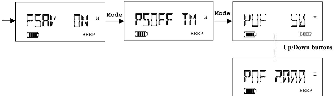
Under the above mode, press Up/Down buttons to select the desired time and then press Mode button or PTT button to set. The radio will then save selection and exit to receiving stand-by mode.
