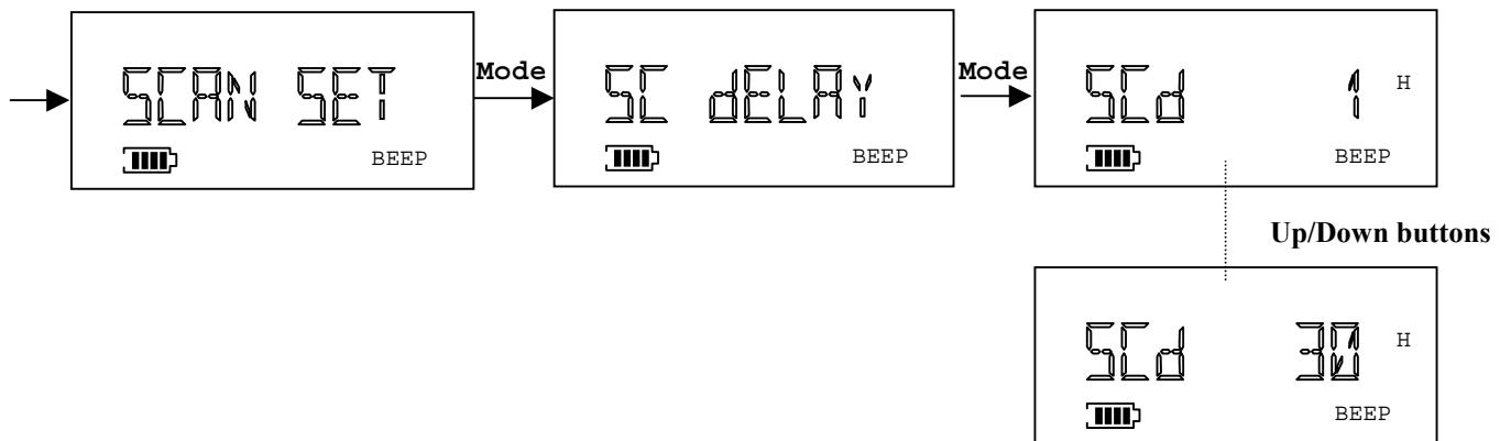
Under the above mode, press Up/Down buttons to select desired time and then press Mode button or PTT button to set. The radio will then save selection and exit to receiving stand-by mode.
