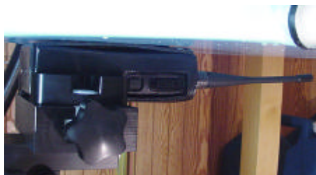
Body-worn SAR Test Setup with 0.9cm Belt-Holster
