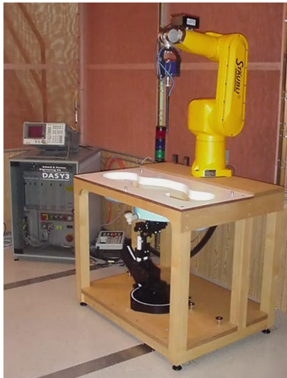
DASY3 SAR Measurement System
