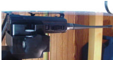
Body-worn SAR Test Setup with 1.0cm Belt-Clip
