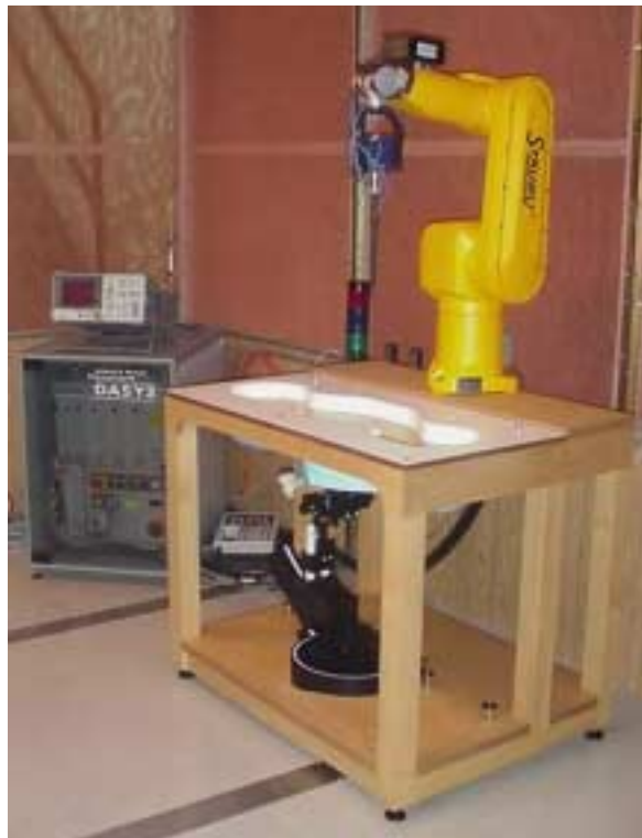
DASY3 SAR Measurement System
