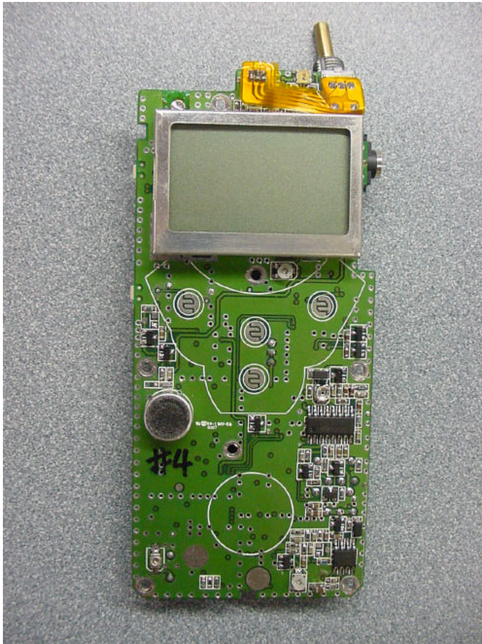
PHOTOGRAPH 17: FRONT OF PCB (MURS-25)
