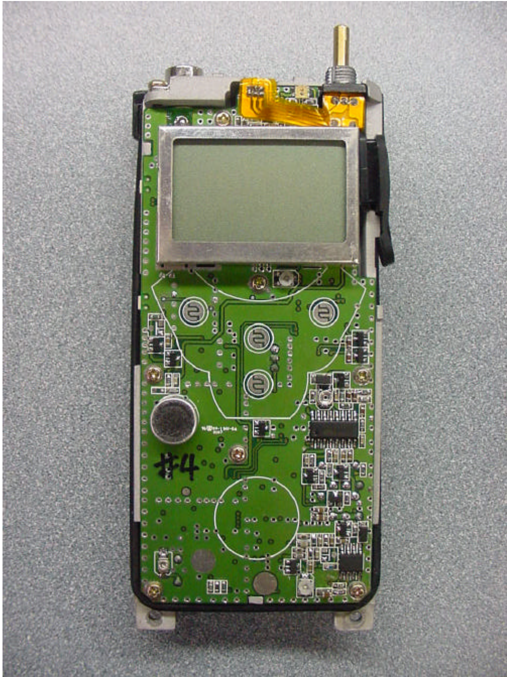
PHOTOGRAPH 12: FRONT OF PCB MOUNTED INSIDE CHASSIS (MURS-25)
