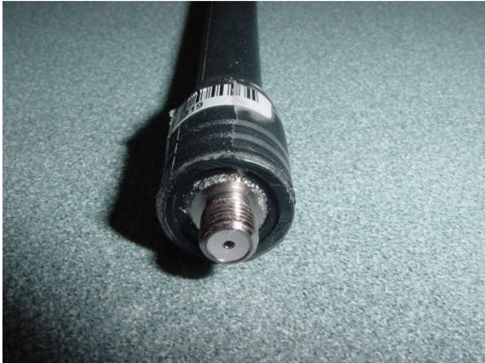
PHOTOGRAPH 34: ANTENNA CONNECTOR (MURS-25)
