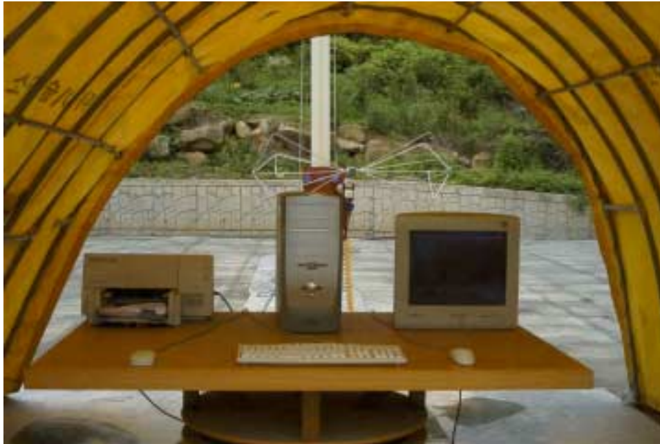
Photograph 1 : Setup for radiated Emissions
