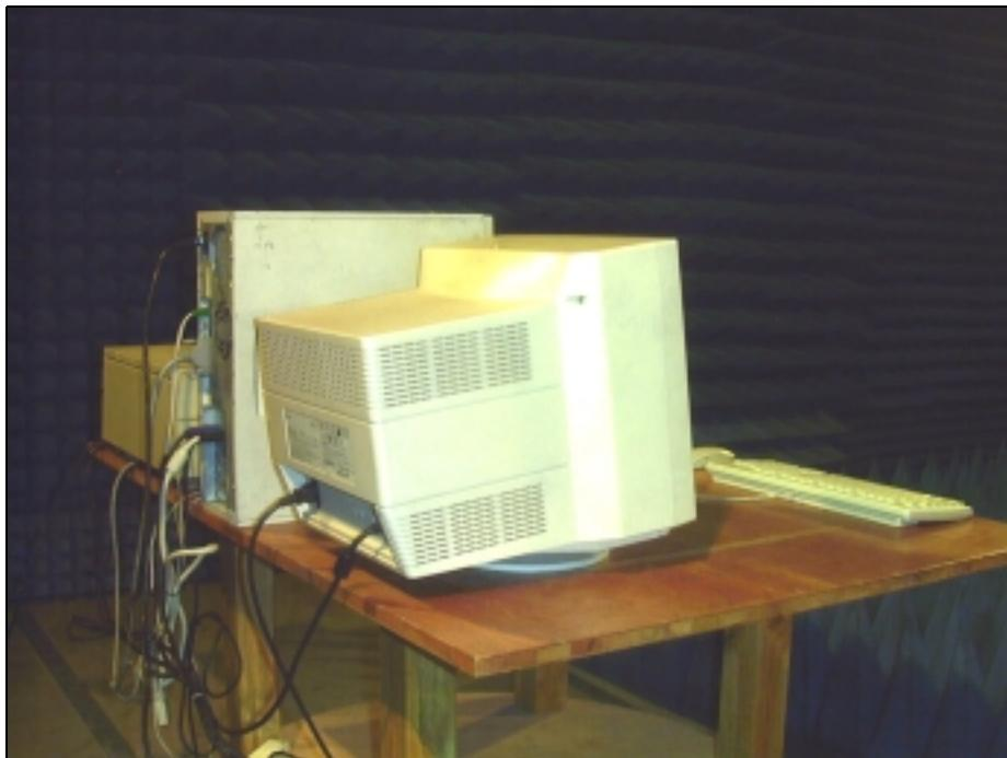
**7.2 Setup with the Maximized RFI Field Strength Emission Level(30-1000MHz)**
