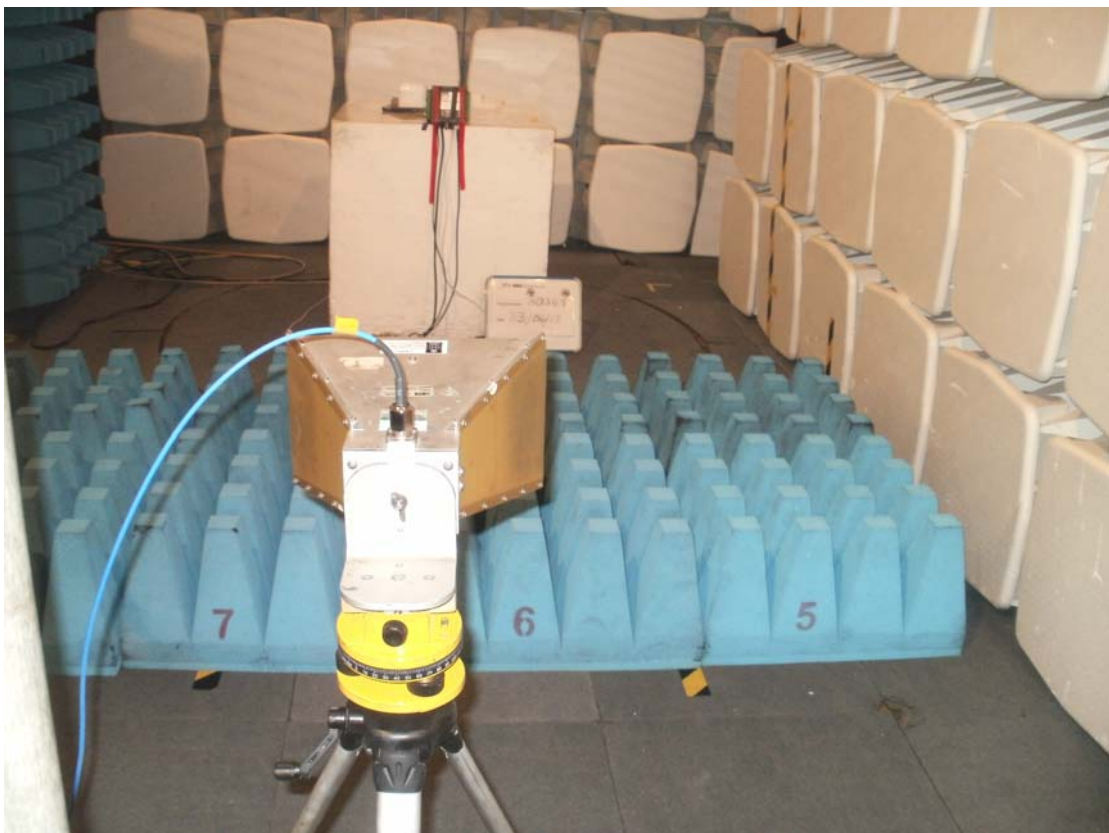
Figure 5.14.6 ICES and FCC Testing Radiated emissions 1GHz to 2GHz in chamber @ 3m
