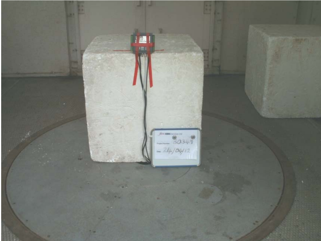
Figure 5.14.7 Canadian & USA Requirements Testing Radiated emissions open area test site 30MHz to 1000MHz @ 10m
