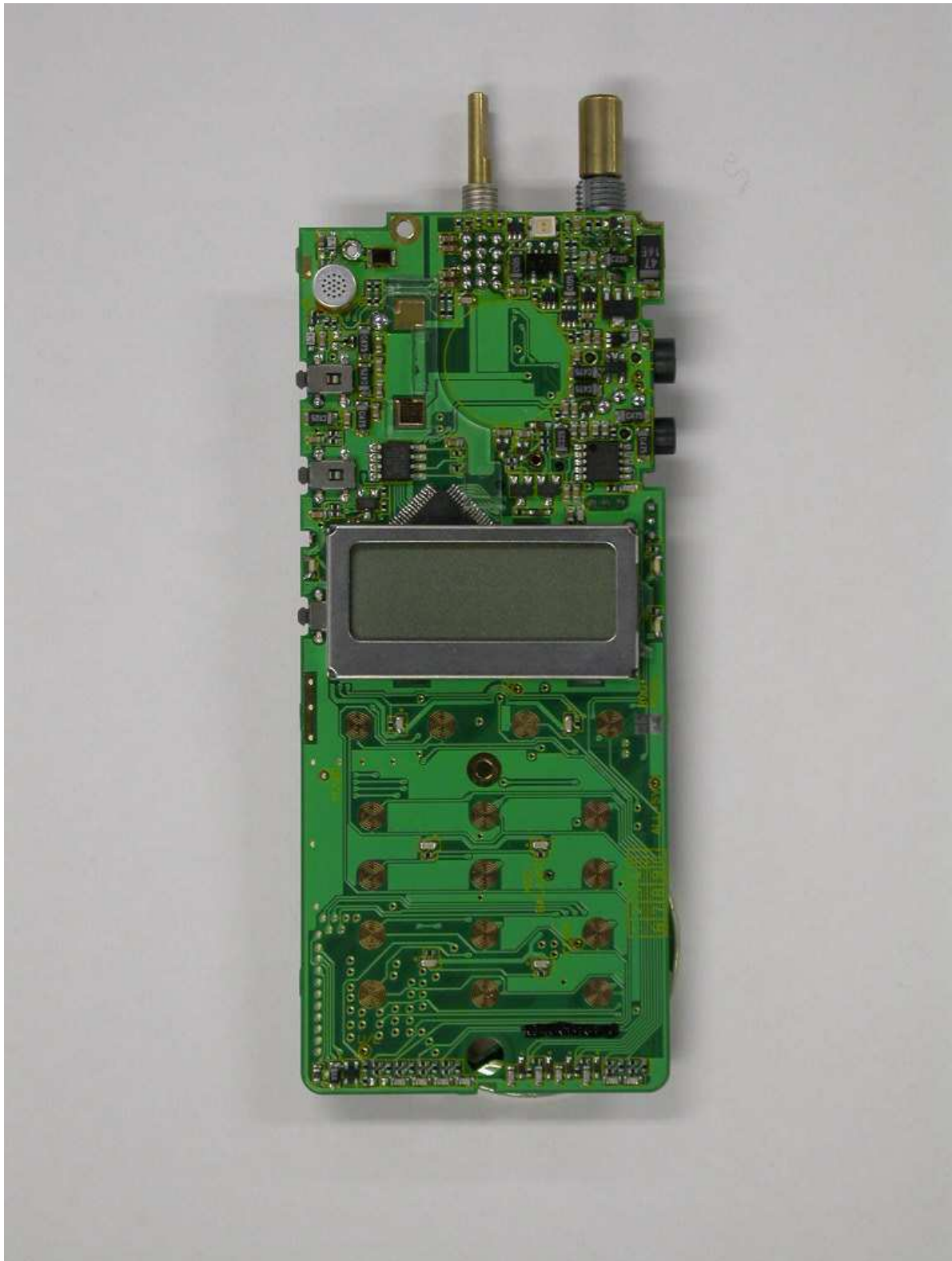
7) MAIN PCB of SC-580 (Component Side View)
