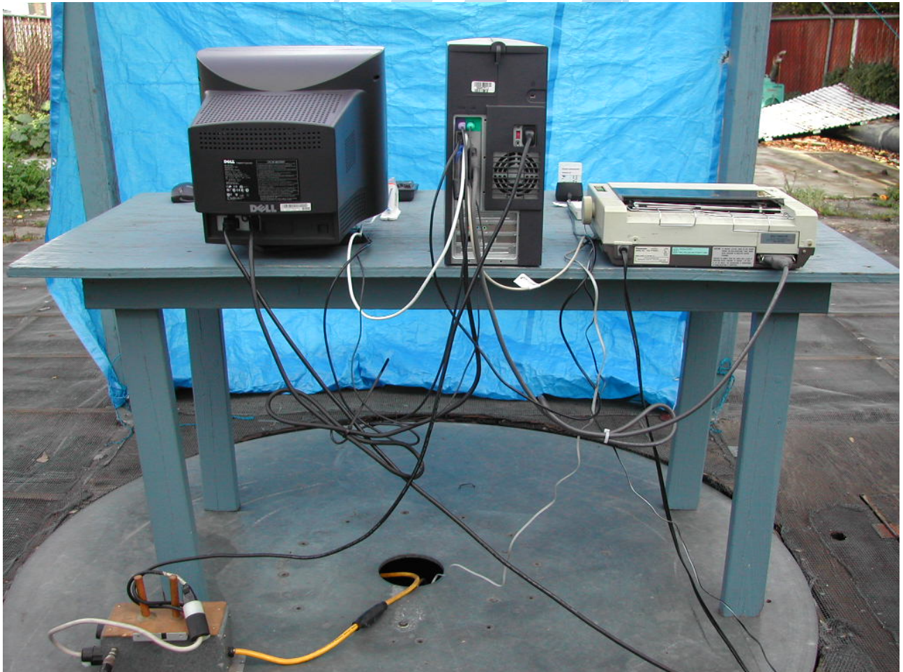
FIGURE 4: PLI Photograph Number 5346C2934SJ-09 illustrates the rear view of the Equipment Under Test with all peripherals attached in conducted Electromagnetic Interference Test Configuration #1 .
