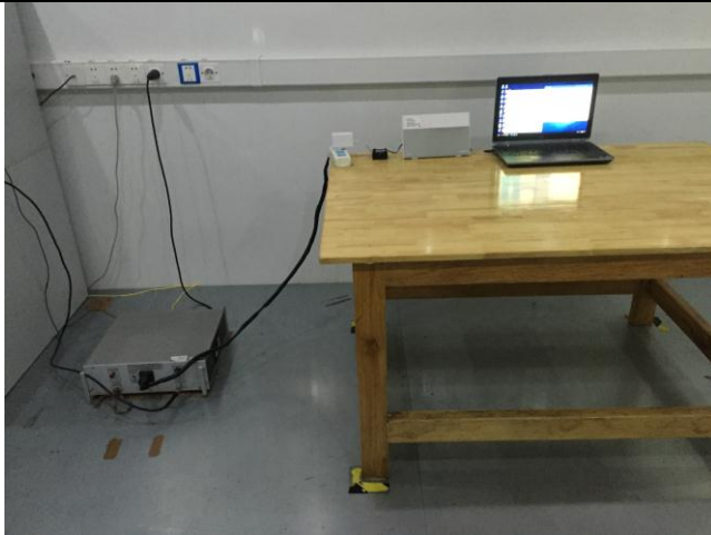
Conducted Emissions Test Setup Front View
