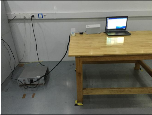
Conducted Emissions Test Setup Front View
