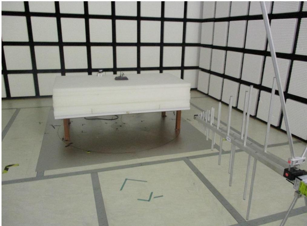
**Radiated Emission Above 1GHz Test**
