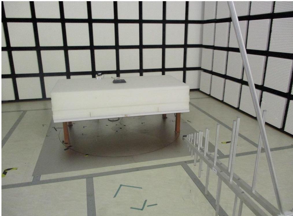
**Radiated Emission Above 1GHz Test**
