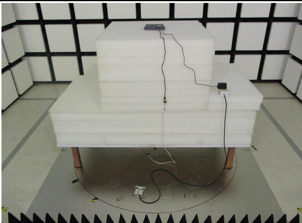
**Radiated Emission Above 1GHz Test**
