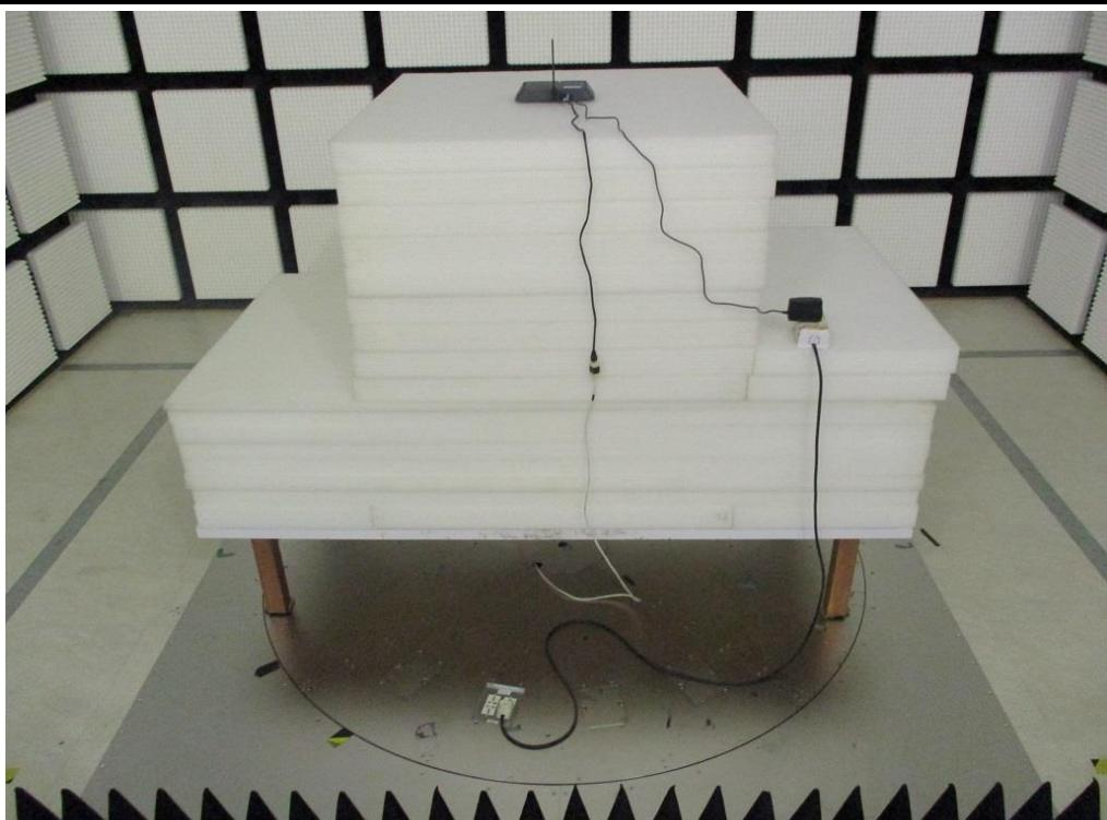
**Radiated Emission Above 1GHz Test**
