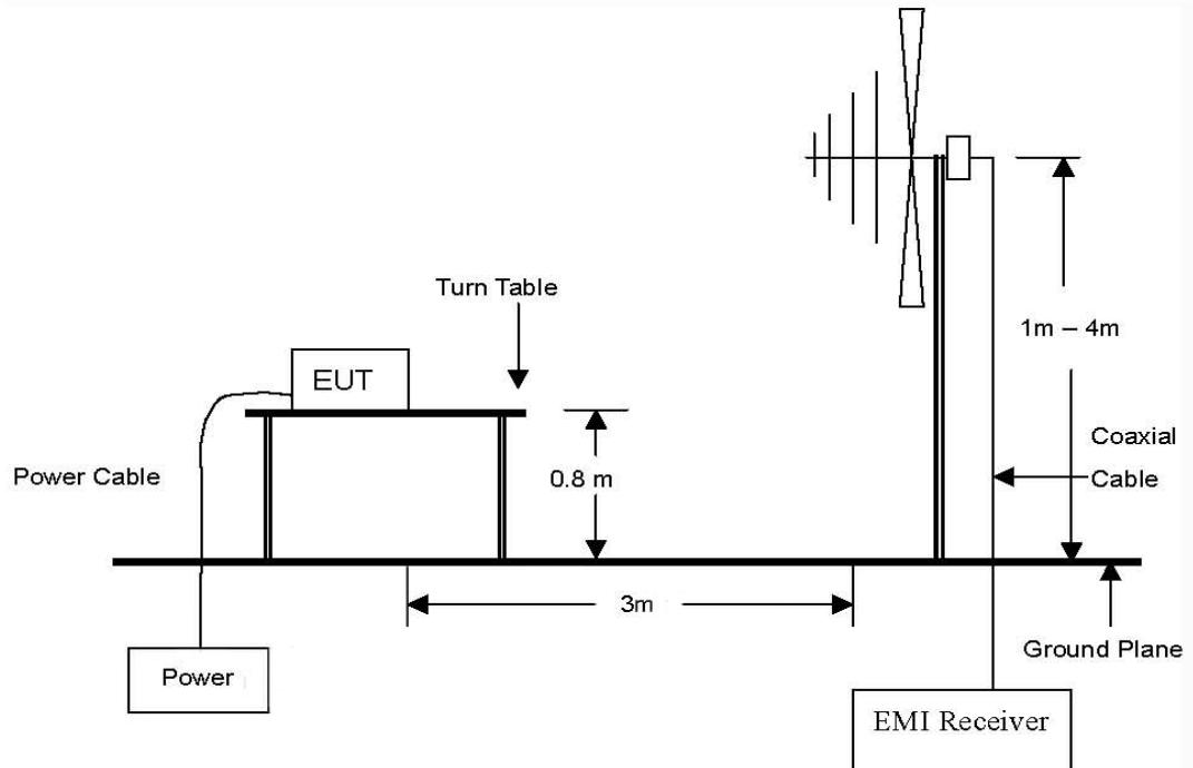
The diagram below shows the test setup that is utilized to make the measurements for emission .The spurious emissions were investigated from 1 GHz to the 10th harmonic of the highest fundamental frequency or 40 GHz, whichever is lower.
