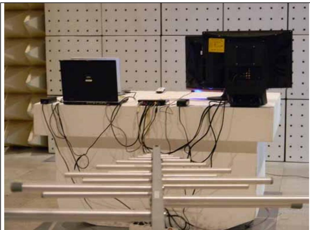
**2.7 Photographs of Radiated Emission (3m method above 1 GHz ~ 18 GHz)**
