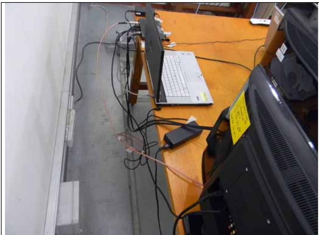
**2.6 Photographs of Radiated Emission (3m method below 1 GHz)**
