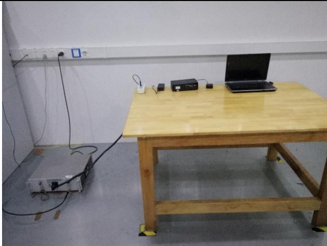
Conducted Emissions Test Setup Front View
