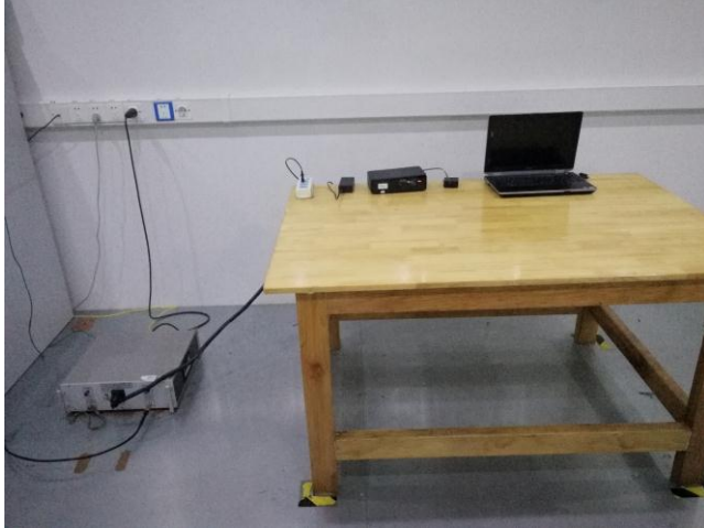
Conducted Emissions Test Setup Front View
