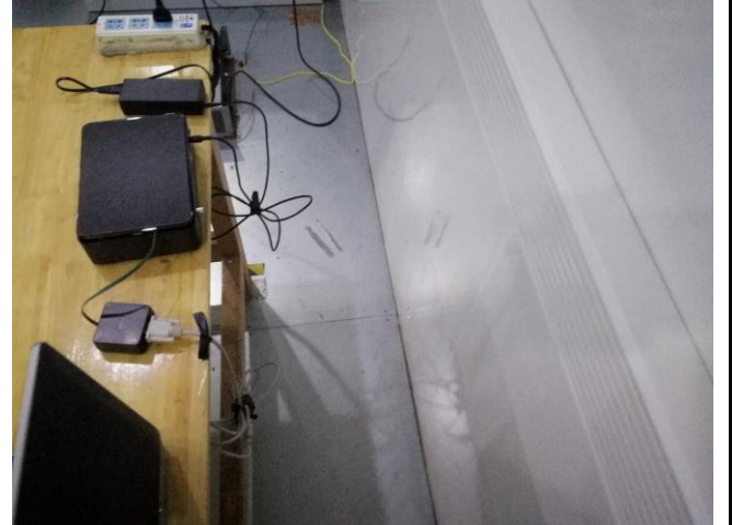
Conducted Emissions Test Setup Side View
