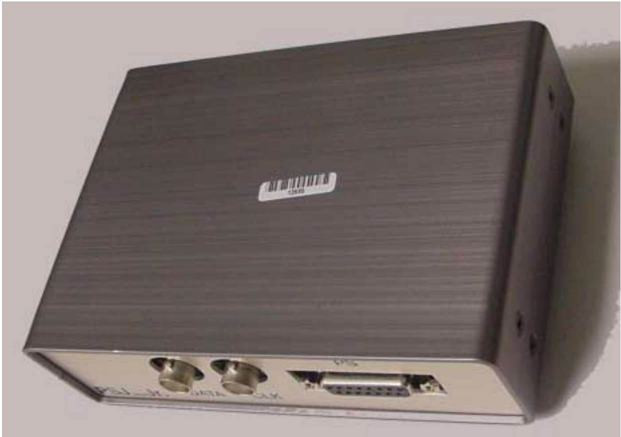
PHOTOGRAPH 24: TOP OF PSJ_JR CONNECTOR BOX
