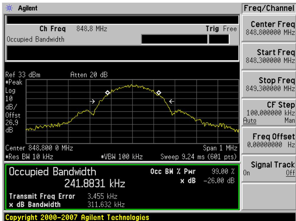
■ GSM1900 MODE (512 CH.) Occupied Bandwidth
