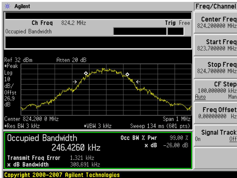
■ GSM850 MODE (190 CH.) Occupied Bandwidth
