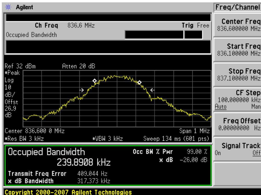
■ GSM850 MODE (251 CH.) Occupied Bandwidth
