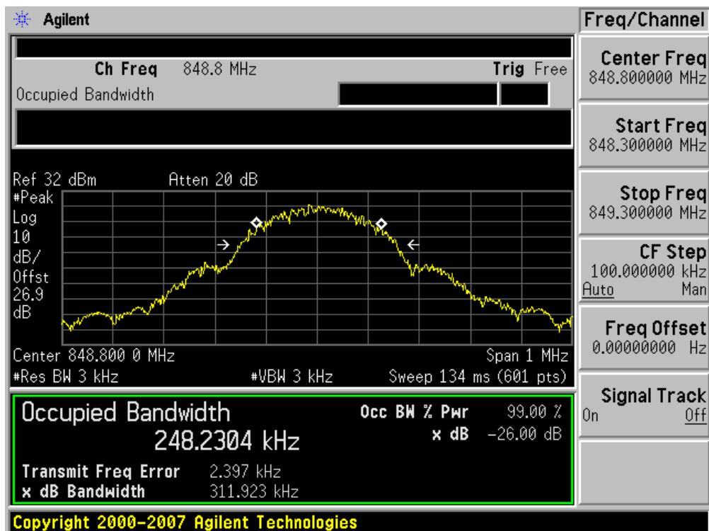
■ GSM850 EDGE (251 CH.) Occupied Bandwidth
