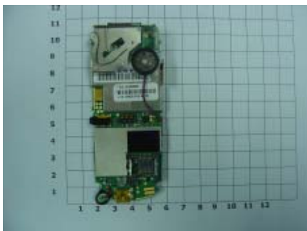
Fig.13 Antenna locations relative to chassis/housing
