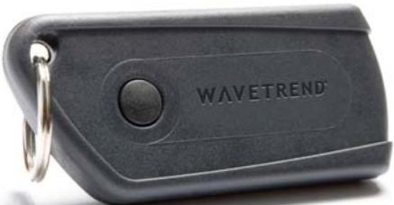
The TG700-A ActivDuo Key Fob PA Tag is an active tag that continuously transmits a unique ID number, which can be detected by Wavetrend® readers. An internal battery powers the tag and Wavetrend's patented ultra low power use design ensures longer battery life at higher rates of transmission than any other brand of active RFID tag. The tag offers immediate alerts on movement.
