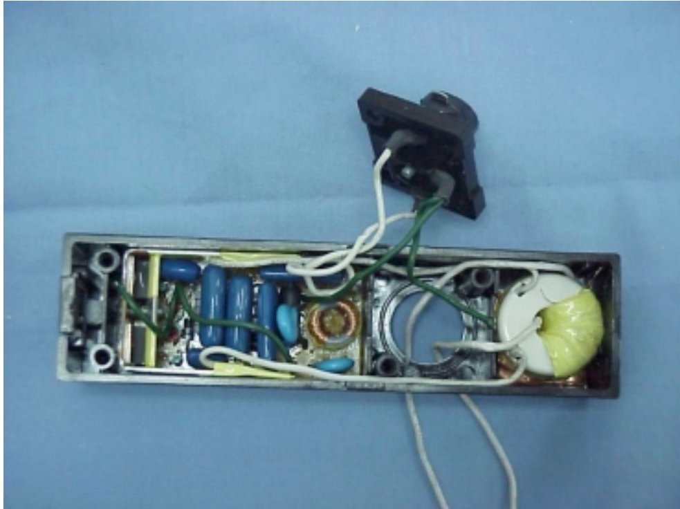
FIGURE 3. POWER SUPPLIES (M/N: 50W) INSIDE VIEW
