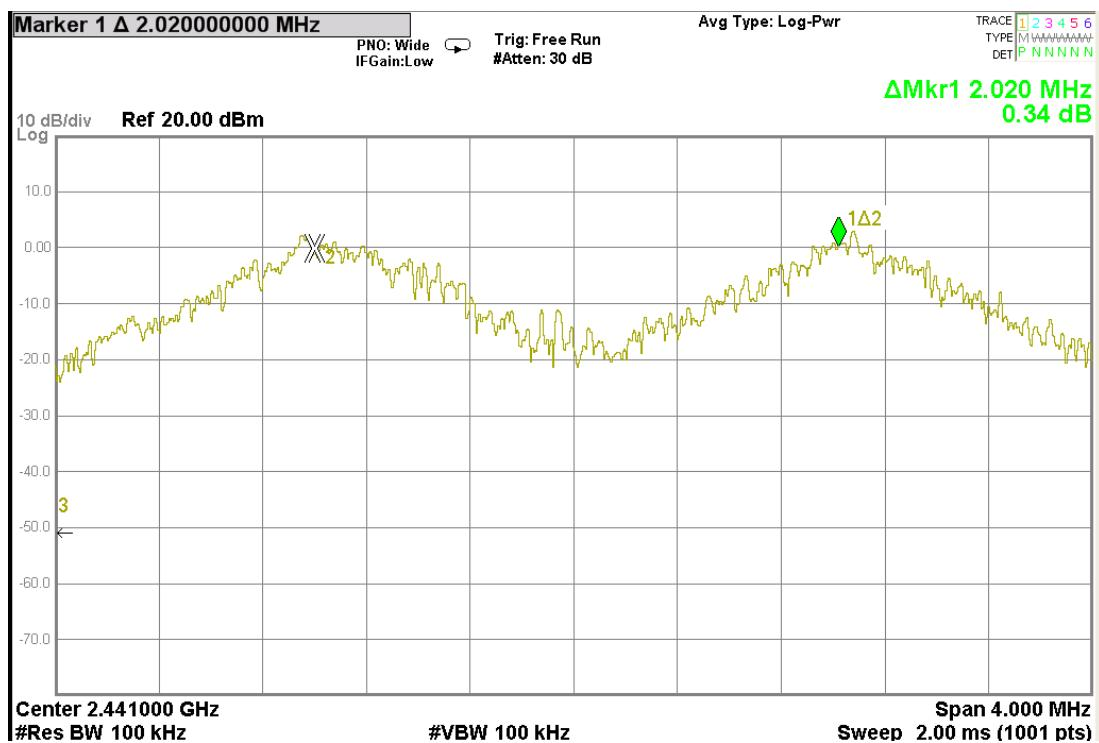
**Carrier Frequency Separation @ Channel 30~31**
