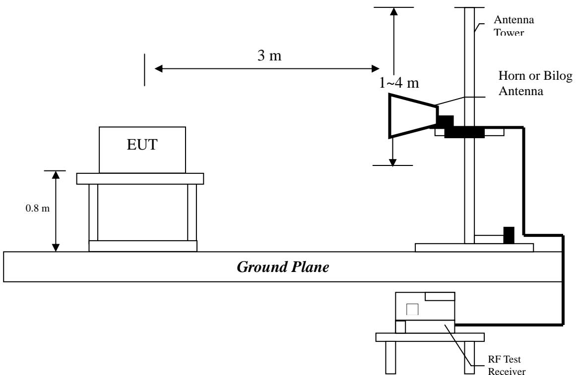
The signal is maximized through rotation and placement in the three orthogonal axes. According to §15.33(a), the spectrum shall be investigated from the lowest radio frequency signal generated in the device, to the tenth harmonic of the highest fundamental frequency or to 40 GHz, whichever is lower. Spectrum Analyzer Resolution Bandwidth is 100kHz or greater for frequencies 30MHz to 1GHz, 1MHz – for frequencies above 1GHz.
