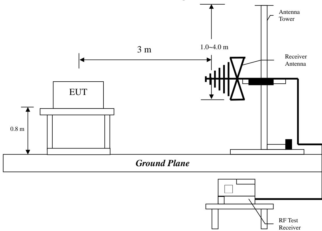
**Radiated emission above 1GHz uses Horn Antenna:**
