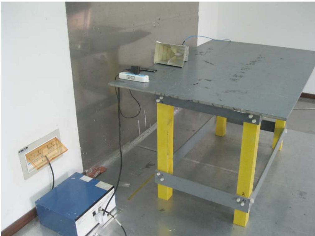
Conducted Emissions Test Setup - Side View
