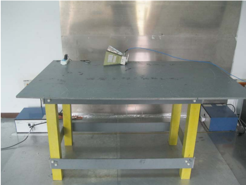
Conducted Emissions Test Setup - Front View
