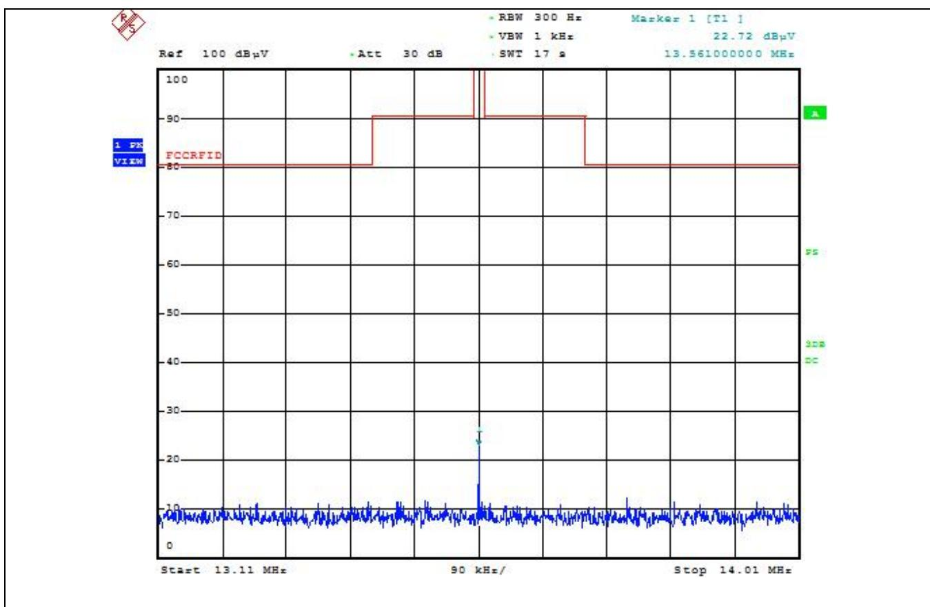
Acc. to above test data, the field strength level of 13.56 MHz is 41.42 dBuV/m and the worst limit subject to 15.225 (b) and (c) is 80.5 dBuV/m, so the EUT meets the requirement.
