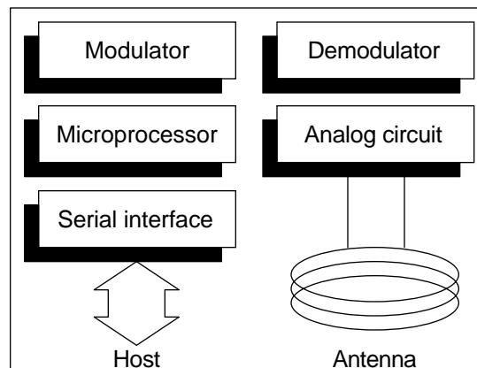
When a read or write command is received, the microprocessor generates a chain of basic commands that are sent to the tag via the modulator and antenna. The tag draws energy from the electromagnetic field created by the antenna and returns an information which is then demodulated and formated before being sent on the serial communication line.
