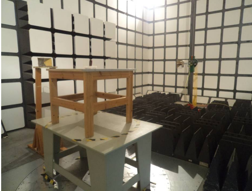
Radiated Emissions Test View
