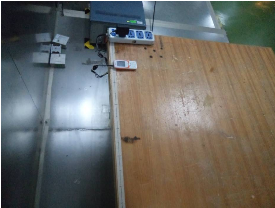
Conducted Emissions - Side View (Charging mode)
