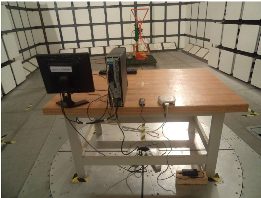
Radiated Emissions – Rear View (downloading mode, 30-1000 MHz)
