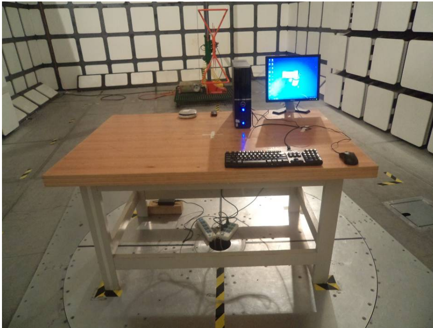
Radiated Emissions-Front View (downloading mode, 30-1000 MHz)
