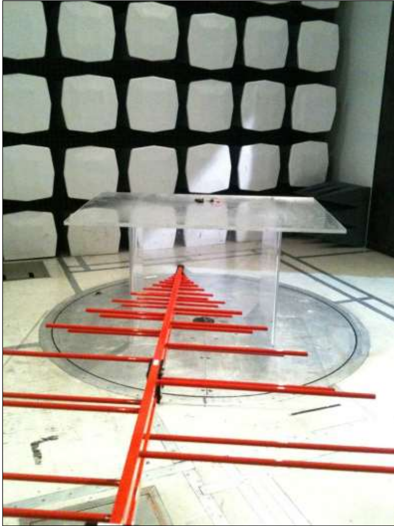
Photograph 1. Radiated Emission Limits Test Setup
