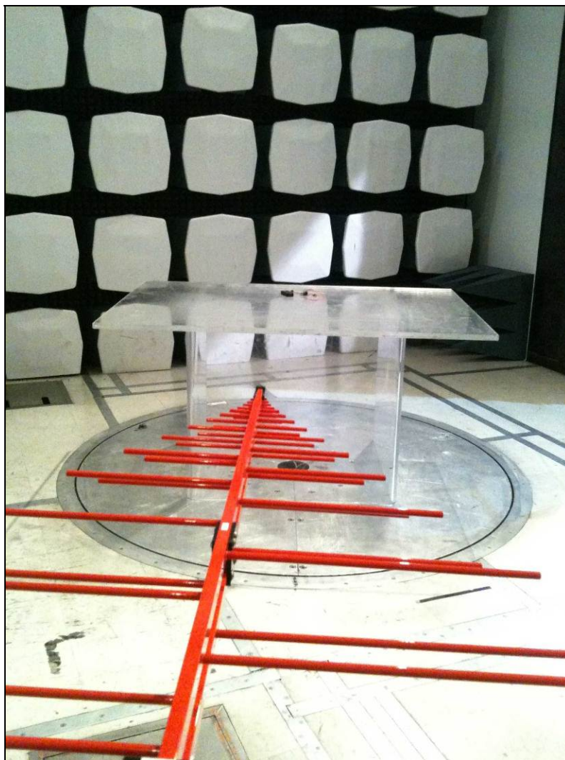
Photograph 1. Radiated Emission Limits Test Setup
