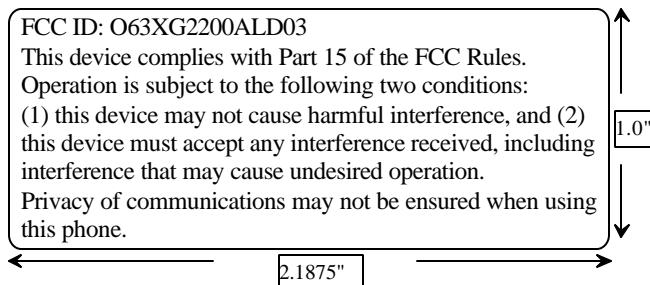
Specifications: Text is black or white in color and is left justified. Labels are silk-screened and shall be “permanently affixed” at a conspicuous location on the EUT.
