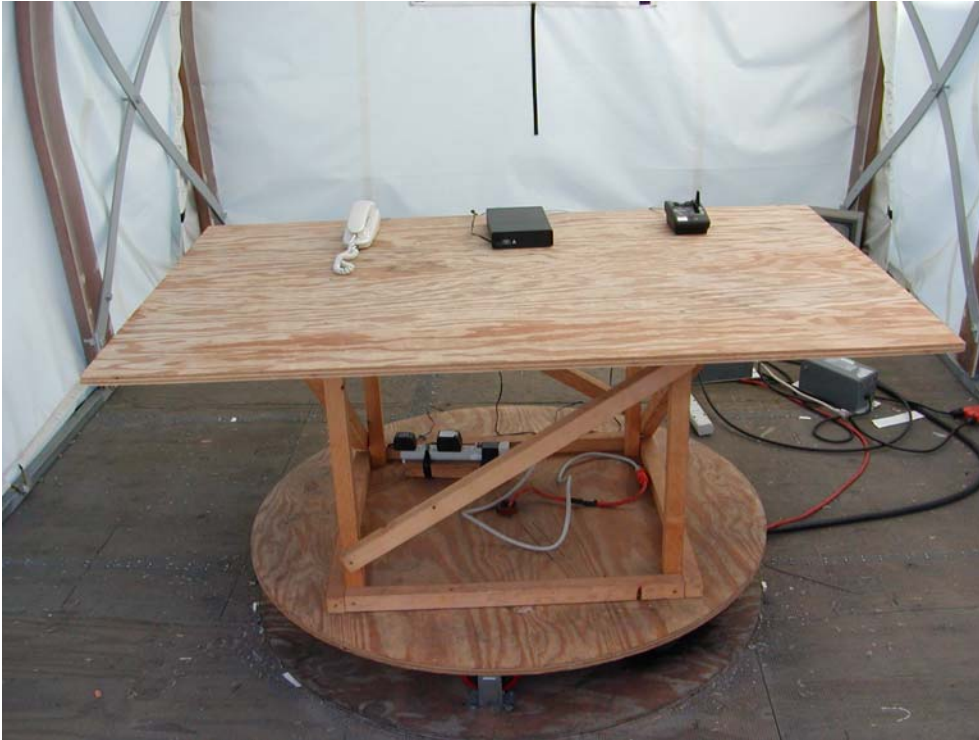
Base Radiated Emission - Front View
