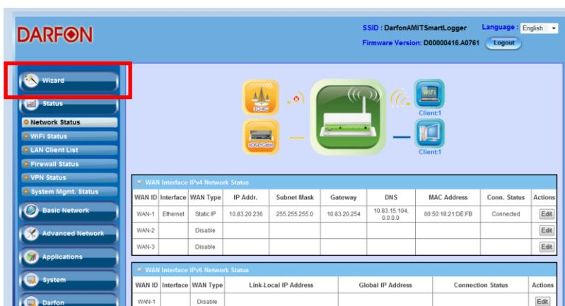
4 The default LAN IP address of this gateway is 192.168.123.254. If you change it, you need to type new IP address.
