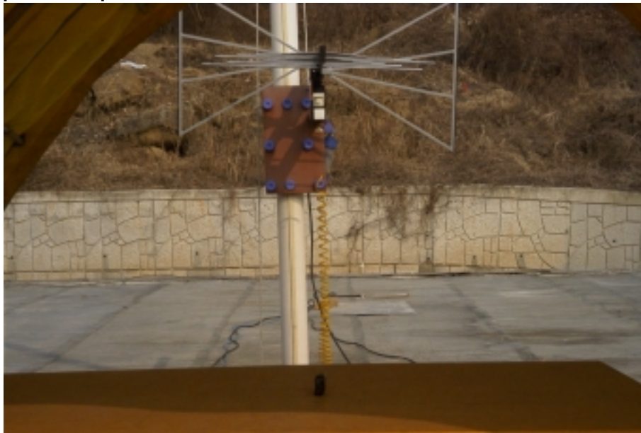
Photograph 1 : Setup for radiated Emissions
