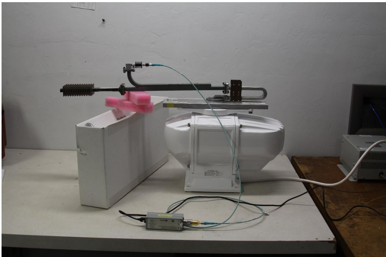
**OCCUPIED BANDWIDTH, SPURIOUS EMISSIONS AT ANTENNA TERMINALS**
