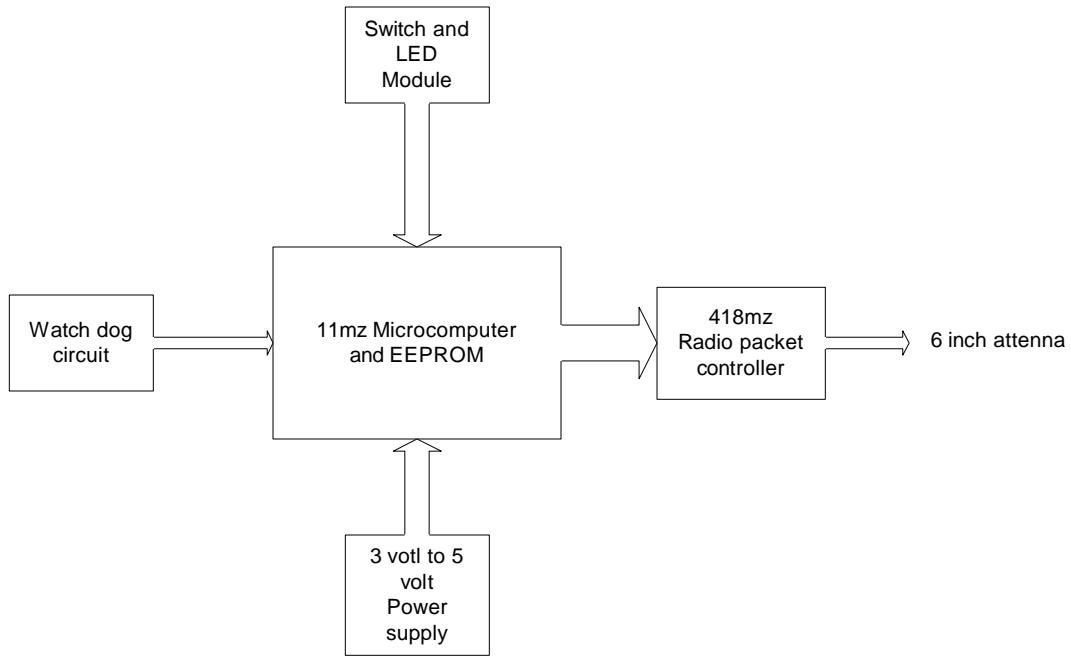
Block diagram of IRC WS1 wireless voting unit
