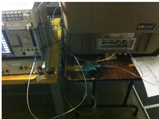
Conducted Output Tests (Power, BW, Spurious)
