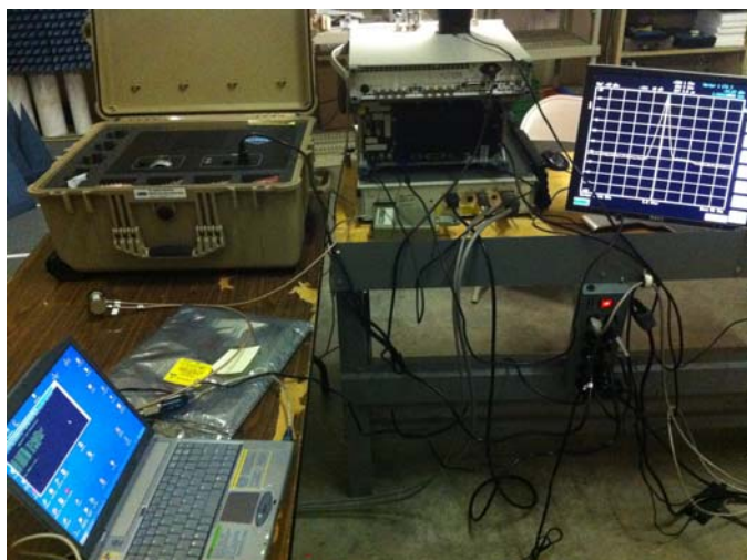
Conducted Output Tests (Power, BW, Spurious)
