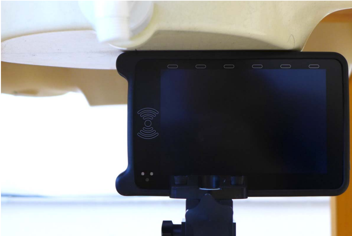
Fig. 20: Top side towards the phantom, 0 mm distance, WWAN antenna.
