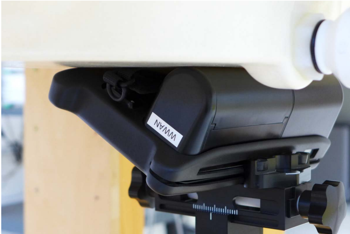
Fig. 22: Back side towards the phantom, 0 mm distance, WWAN antenna.
