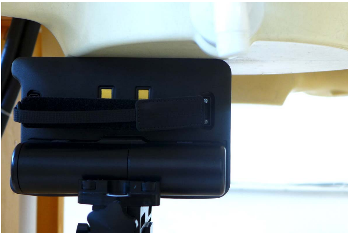
Fig. 23: Bottom side towards the phantom, 0 mm distance, BT antenna.
