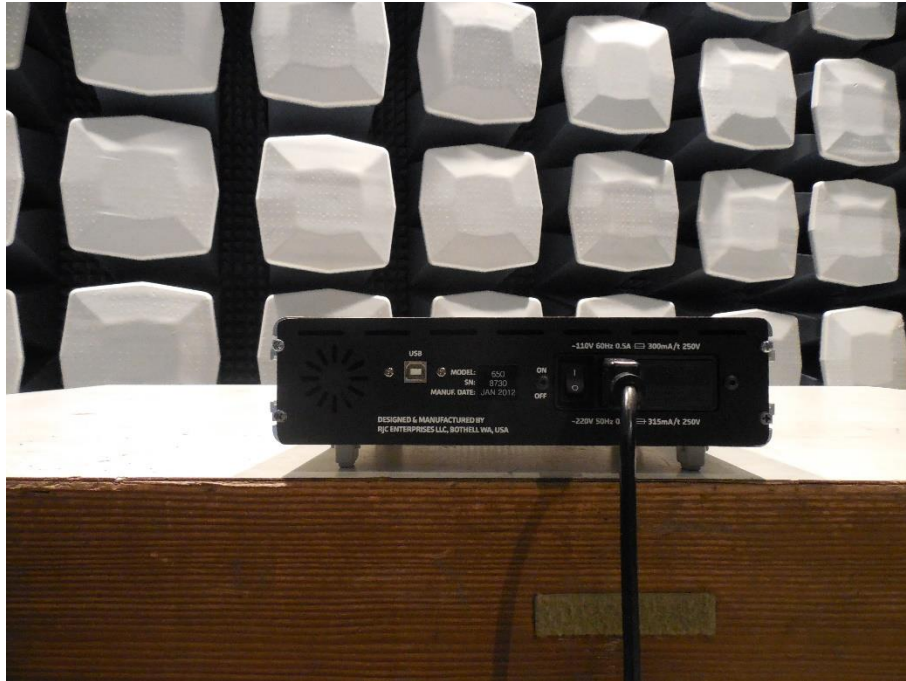
Radiated Emission (close-up view) Test Setup
