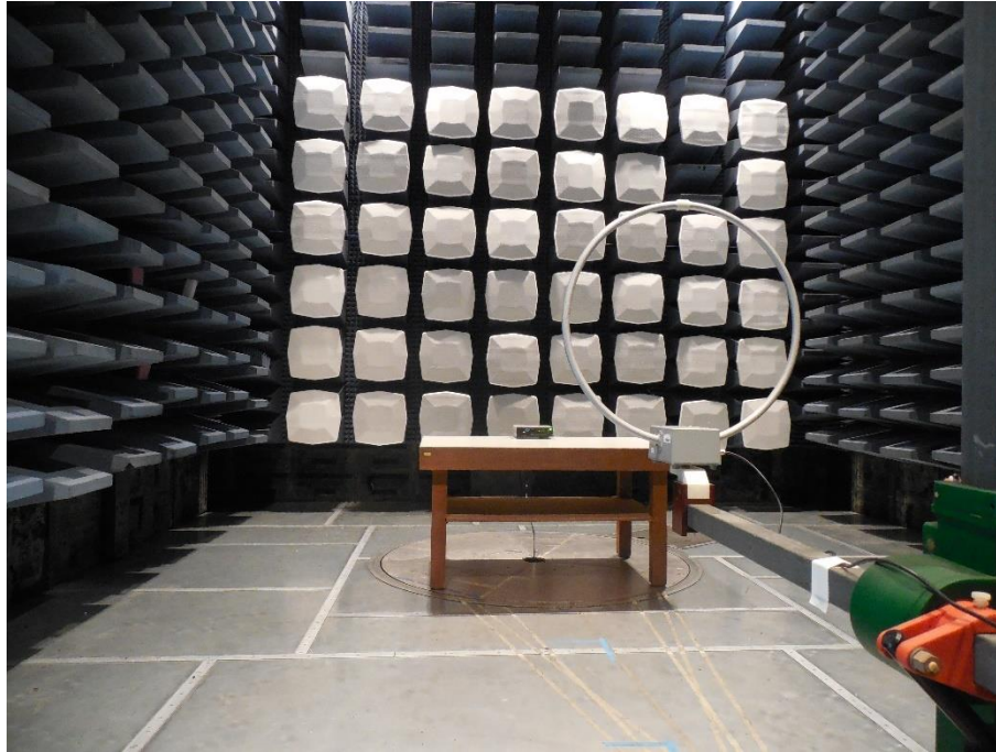
Radiated Emission Test Setup, below 30MHz
