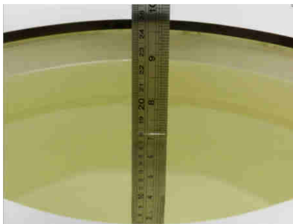
Fig 10.1 Photo of Liquid Height for Body SAR
